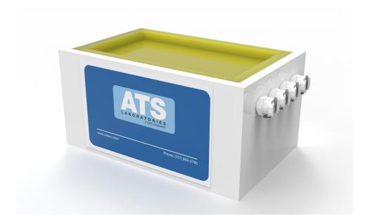
The ATS Model 524 tissue mimicking Doppler flow phantom contains four flow channels simulating superficial vasculature. The simulated vessels are located 15 mm below the scan surface. Built-in scanning wells are provided to permit the use of water or a low viscosity gel as acoustic coupling agents.
